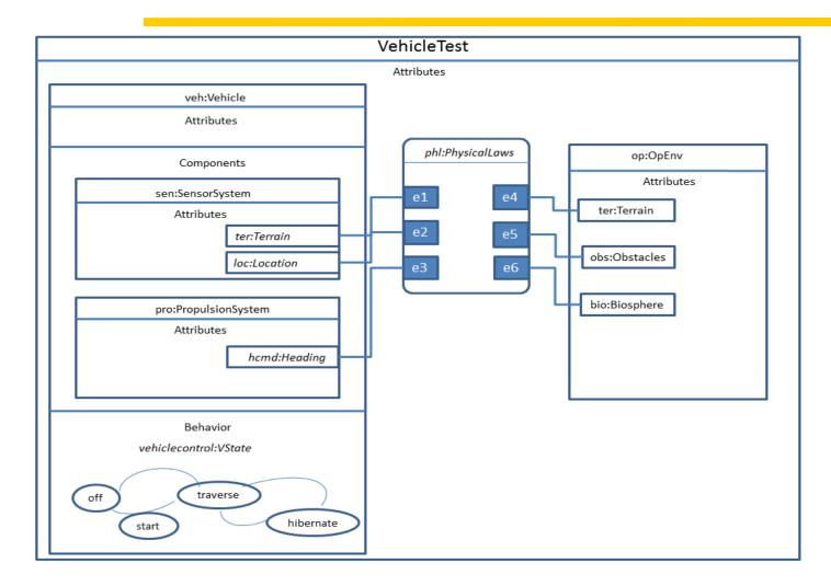
This a view of a SysML vehicle test model used to generate the simulation. The behavior is described by state charts.
